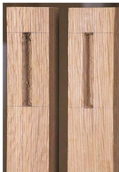
Here's the finished results of using a mortising machine (left) and a hand cut mortise (right). The hand-chopped mortise is prettier, right?
