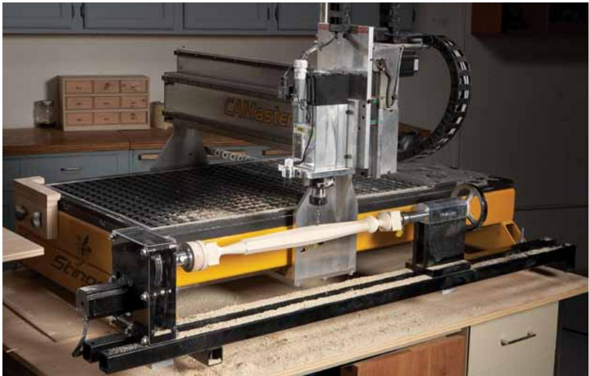
**A ROTARY INDEXING HEAD** allows a CNC machine to create 3-dimensional shapes in the round. It's an accessory that can be added to most CNC machines. Some companies even make it as a stand alone machine. A rotary indexing head looks similar to a standard woodturning lathe, but its approach to shaping wood is quite different. In fact, it's more like milling than woodturning. One of the best features of a rotary indexing head is its ability to create shapes that aren't easily turned on a standard
