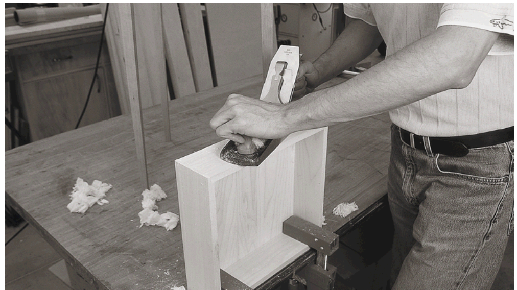
Next, a larger jack plane removes material from both sides until the drawer slides in smoothly.
