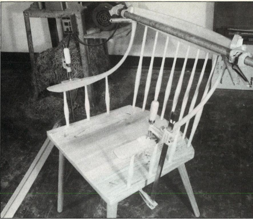
**Glue the arms to the back rail with the spindles dry-assembled in place. Wedges with a 10° taper help the clamps apply even pressure.**
