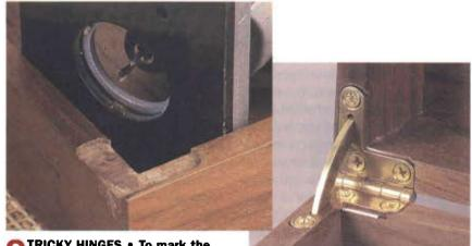
**9**TRICKY HINGES • To mark the hinge location, place it flush to the inside corner on both sides and
