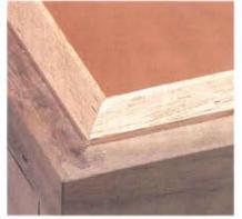
**2** THE FINISHED JOINT • This detail photo shows the assembled joint with cedar lining in place. Note the bevel cut on the top edge of the cedar lining. This detail plays an important role in providing an airtight seal for the lid.
