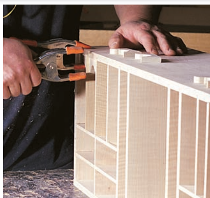
The insert is merely slid into the desk after finishing. You don't need to attach it to the lower case if you don't want to. Here I'm fitting the pigeonhole scrollwork into the cubbyholes using spring clamps.
