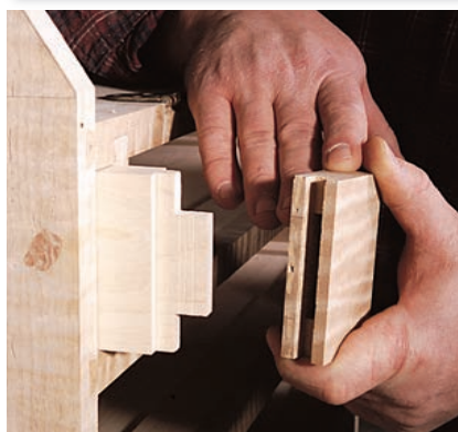
The support end on the lid support, (attached with a haunched mortise), is a nice way to conceal the end grain.
