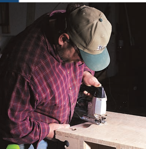
Here you can see how I build my bases. I add a block at the front and attach the moulding to that. It's much like a kick on a traditional cabinet, except it's flush to the front of the case. Cut out the scroll pattern using a jigsaw (top). After you've cut out the scroll pattern on the ogee feet, nail them in place to the sides and the block at front (right).
