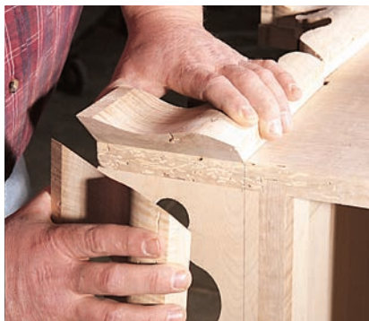
Here you can see how I build my bases. I add a block at the front and attach the moulding to that. It's much like a kick on a traditional cabinet, except it's flush to the front of the case. Cut out the scroll pattern using a jigsaw (top). After you've cut out the scroll pattern on the ogee feet, nail them in place to the sides and the block at front (right).
