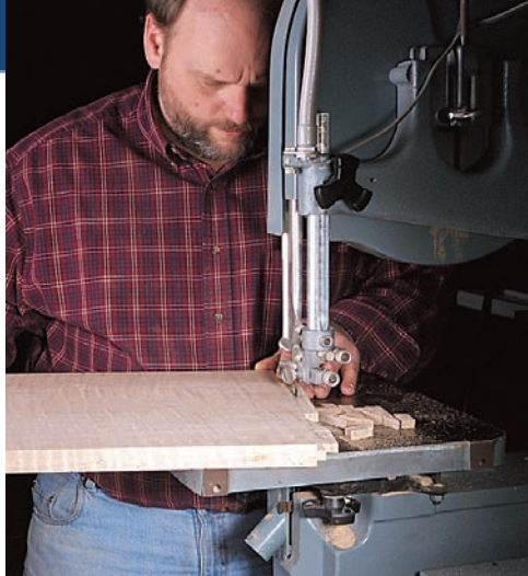
Cut the tails on your band saw and clean them up with a chisel if necessary.
