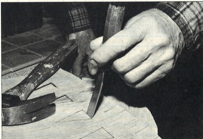
On the other end of the piece, he cuts the shape that will receive the fingers.
