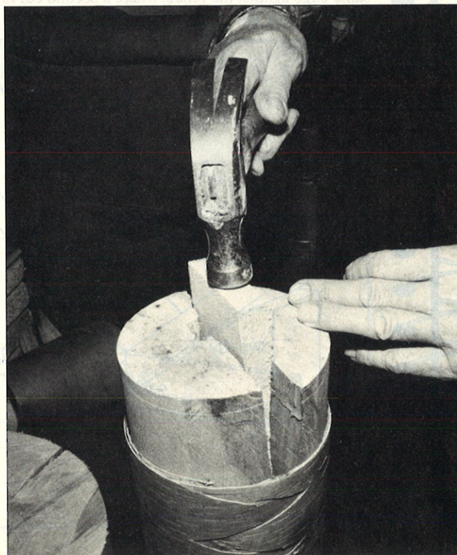
He puts the glued bark onto a tree core that has been split in half, then he drives wedges tightly into each end and lets it dry.
