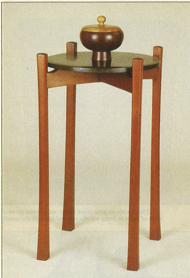
An aniline dye was used to achieve the brilliant red color on the mahogany legs of this contemporary table. (Table by the author, top of African wenge)
