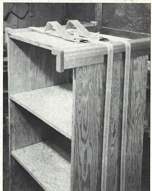
The Lamello Spanner Set includes aluminum extrusions that fit on the corners of a carcass.
